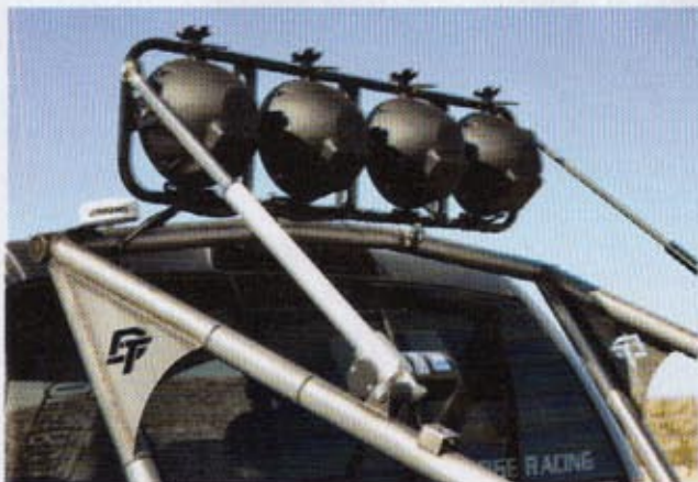
▲ Here is a closer look at the lightbar mounting. The driver side of the lightbar is controlled with a linear actuator hooked to a switch in the cabin. The passenger side has a strut mounted to keep vibration down.
