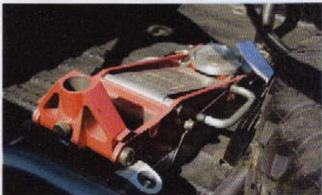
▲ Dirt-Tech sells this handy aluminum floor-jack mount which can be mounted to any truck bed or custom-mounted if you choose. The jack slides in and locks itself in place. You may add a keylock if you are worried about theft. Having a fullsize jack is a must when owning a tall truck, unless you feel like calling AAA every time you get a flat. The stock jack just won't cut it.
